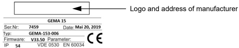
Figure 8: Example of a type plate for a GEMA controller box
