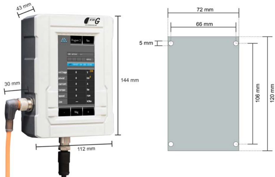
Figure 11: Dimensions of the HMI control unit and the metal plate
