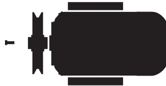
Figure 14: Installation of the belt pulley
